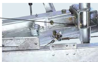
Support roue jockey montage central
